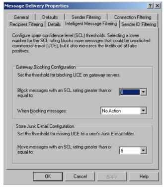
Figure 4: IMF integration in Exchange Server SP2
