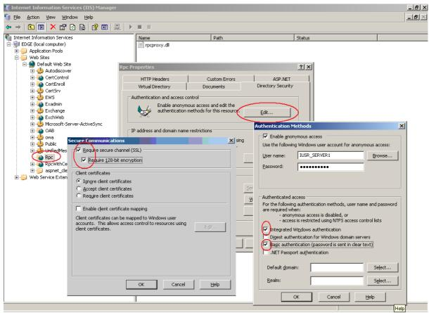
Figure 4: Enable SSL and Authentication
