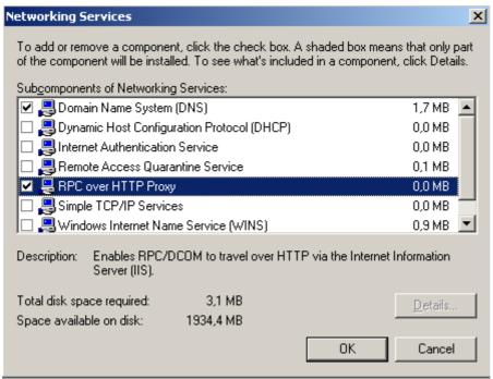
Figure 1: Install the RPC over HTTPS Proxy
