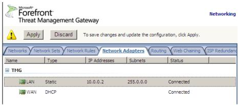
Figure 7: Network Adapter configuration in TMG
