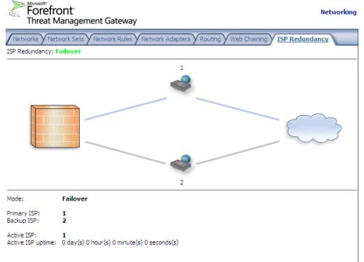
Figure 10: ISP Failover Redundancy GUI
