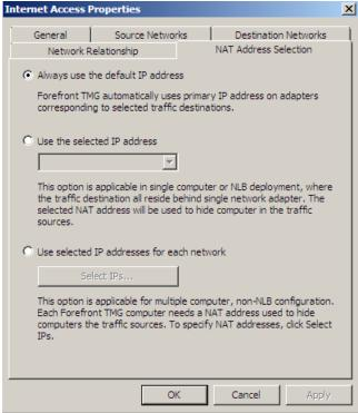
Figure 6: Network Address Translation based on TMG networks
