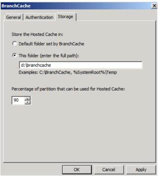
Figure 4: Select the location for BranchCache content and the Percentage of disk space used for Hosted Cache.
