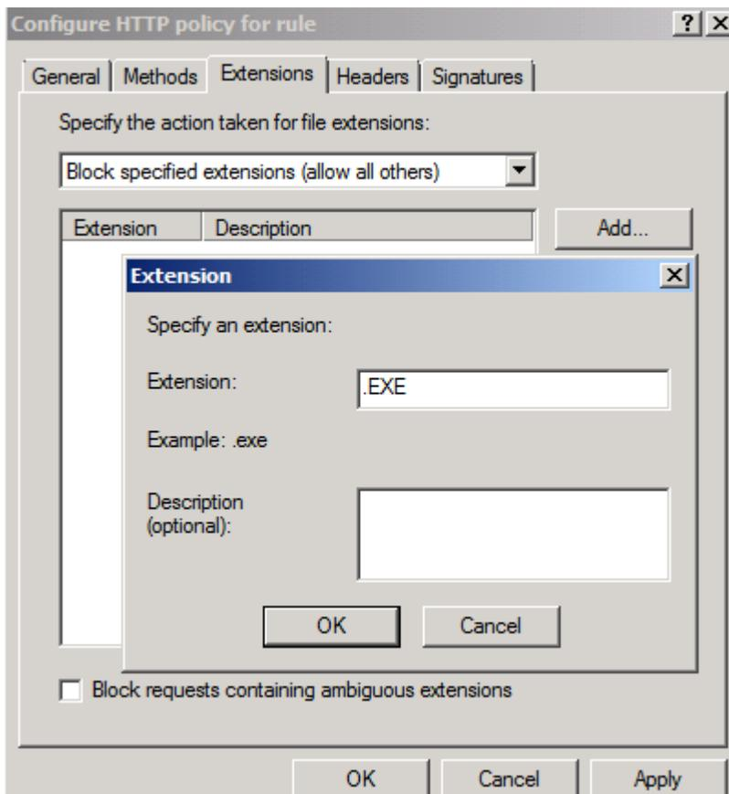
Figure 4: Using Forefront TMG to block downloading files with the EXE extension
